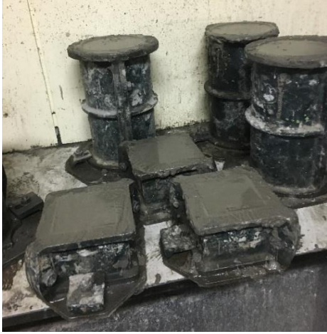
Figure 5.1: Wet concrete in moulds
