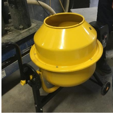
Figure 8.1: Concrete mixing drum
