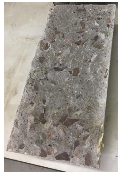
Figure 8.8: Half of plain concrete cylinder after splitting test
