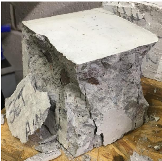
Figure 8.7: Plain concrete cube after compression test
