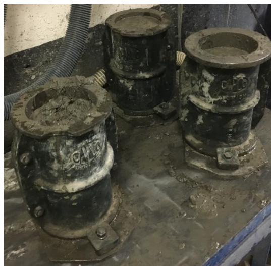
Figure 8.3: Concrete tamping on vibrating table
