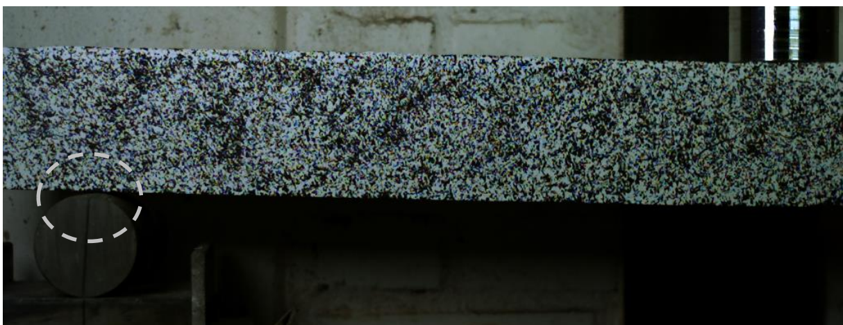
Figure 6.14 Response of RPC2 after 2.0 ms, when the maximum lift occurs over the support.
