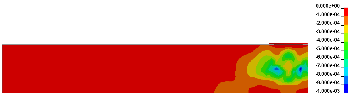
Figure 6.25 3 rd principle strain (compression) 0.07 ms after impact.
