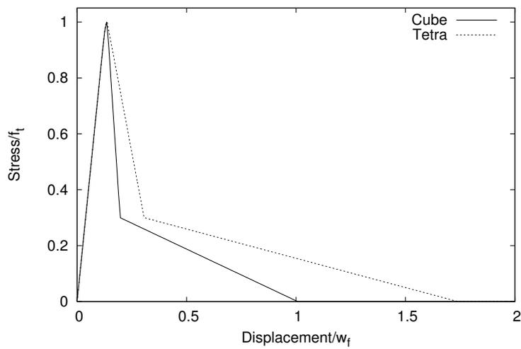
Figure 10: Comparison of Stress-displacement curves for a single brick and tetrahedron using MAT\_CDPM together with the explicit analysis.
