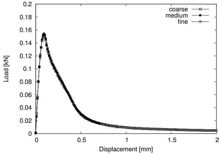
Figure 7: Load versus displacement for three hexahedral meshes using MAT\_CDPM together with the explicit analysis.
