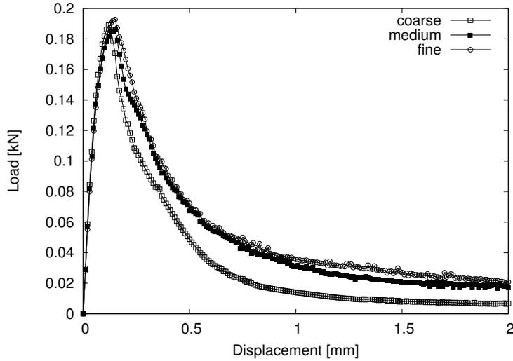
Figure 5: Load versus displacement for three tetrahedral meshes using MAT\_CDPM together with the implicit analysis.
