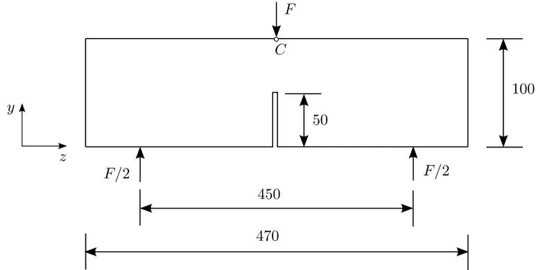
Figure 1: Three point bending test: Geometry and loading setup. The notch thickness is 5 mm.
