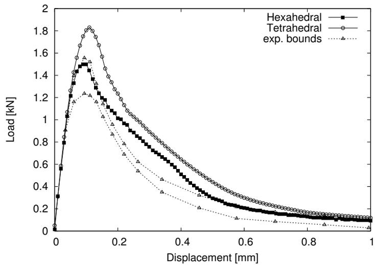
Figure 8: Comparison of Load-displacement curves for the coarse hexahedral and tetrahedral meshes using MAT\_CDPM together with the explicit analysis.
