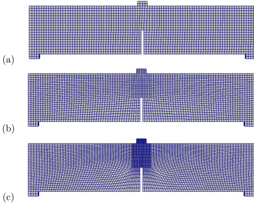
Figure 6: Three point bending test: Coarse, medium and fine hexahedral meshes.
