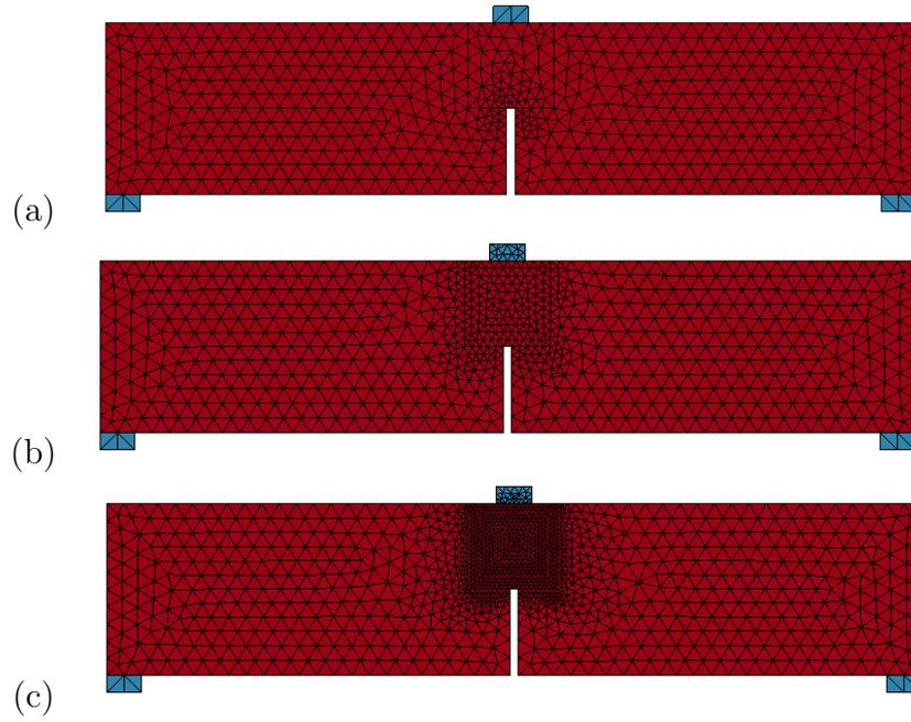
Figure 3: Three point bending test: Coarse, medium and fine tetrahedral meshes.
