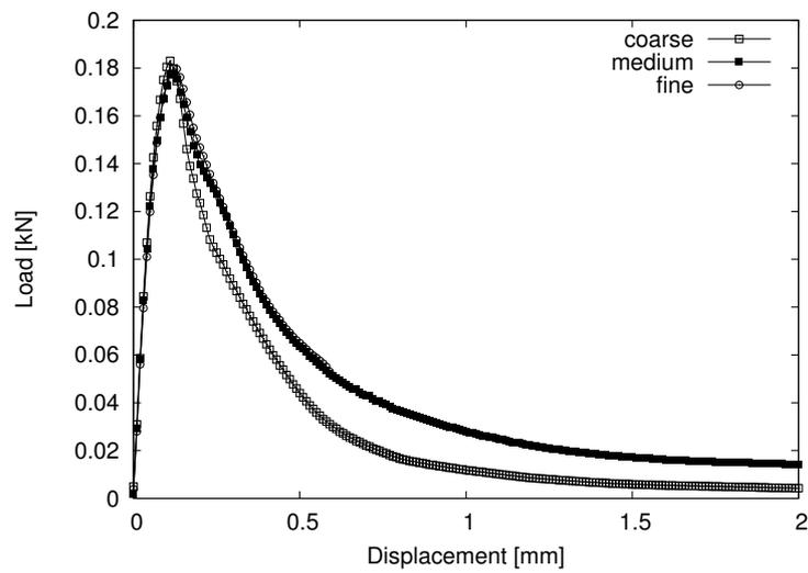
Figure 4: Load versus displacement for three tetrahedral meshes using MAT\_CDPM together with the explicit analysis.
