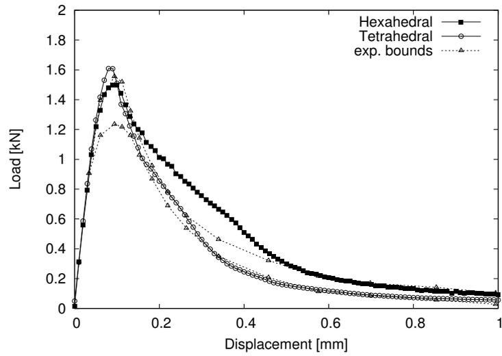
Figure 11: Comparison of Load-displacement curves for the coarse hexahedral and tetrahedral meshes using MAT\_CDPM with the modified input for the tetrahedral mesh using the explicit analysis technique.
