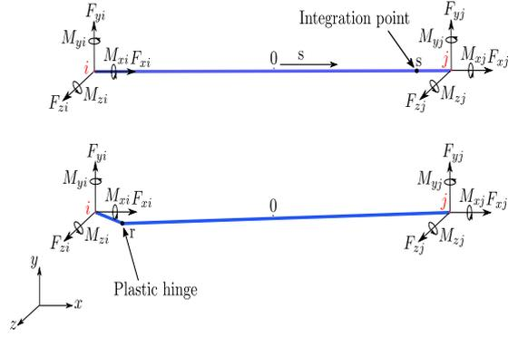
Figure 2: Linear Timoshenko beam element with the option to shift integration points [9].
