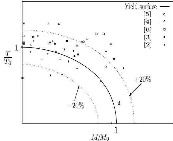
Figure 4: Comparison of torsion-moment interaction of the model and experiments reported in the literature.
