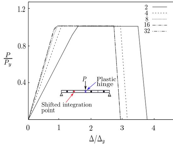
Figure 3: Effect of mesh-refinement on the load-displacement curve.
