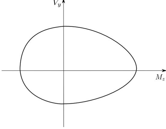
Figure 1: The ellipsoidal strength envelope for four quarter-ellipsoidal shear-moment interaction curves with different limits for shear and moment.
