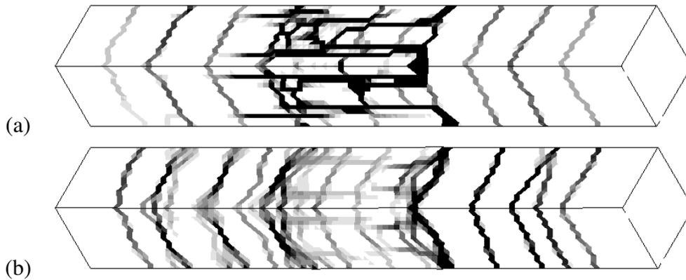
Figure 3: Contour plots of the maximum principal strain for lab splices (a) without fibres and (b) with fibres. Black indicates strains which correspond to crack openings greater than 0.3 mm.
