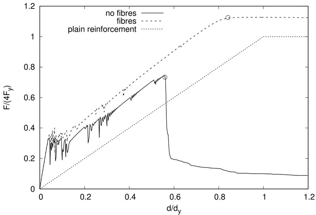
Figure 2: Load-displacement curves for straight reinforcement laps in concrete with a lap length of  $L_s = 500 \text{ mm}$  with and without fibres obtained from nonlinear finite element analyses with the concrete damage plasticity model CDPM2.
