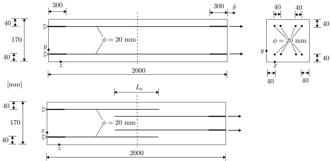
Figure 1: Geometry of the lab splicing in direct tension. The specified dimensions refer to the centre lines of the reinforcement bars.
